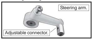
Adjust the nose gear steering arm until the arm is parallel with the fire wall.
