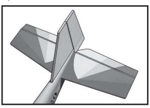
☐ 3) While holding the vertical stabilizer firmly in place, use a pen and draw a line on each side of the vertical stabilizer where it meets the top of the fuselage.
