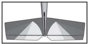
☐ 8) After the epoxy has fully cured, remove the masking tape or T-pins used to hold the stabilizer in place. Carefully inspect the glue joints. Use more epoxy to fill in any gaps that may exist that were not filled previously and clean up the excess using a paper towel and rubbing alcohol.
