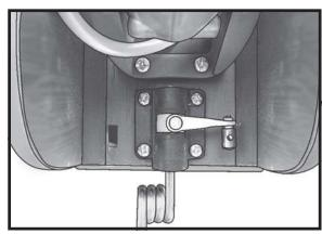
Install the pushrod wire as shown.
