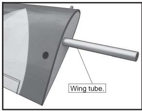
☐ 2) Remove the brace when satisfied with its fit ineach wing half. Coat both sides of one half of the dihedral brace with 30 minute epoxy. Next, pour some epoxy into the dihedral box in one wing panel. Make sure you cover the top and bottom as well as the sides of the dihedral brace. Use enough epoxy to fill any gaps.
