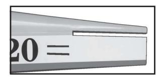
□1) Using a ruler and a pen, locate the centerline of the horizontal stabilizer, at the trailing edge, and place a mark. Use a triangle and extend this mark, from back to front, across the top of the stabilizer. Also extend this mark down the back of the trailing edge of the stabilizer.
