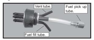
When the stopper assembly is installed in the tank, the top of the vent tube should rest just below the top surface of the tank. It should not touch the top of the tank.
