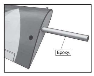
Carefully slide the two wing halves together and firmly press them together, allowing the excess epoxy to run out. There should not be any gap in the wing halves. Use rubbing alcohol and a paper tower to clean up any excess epoxy.
