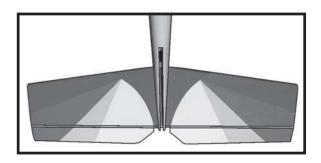
☐ 4) With the stabilizer held firmly in place, use a pen and draw lines onto the stabilizer where it and the fuselage sides meet. Do this on both the right and left sides and top and bottom of the stabilizer.
