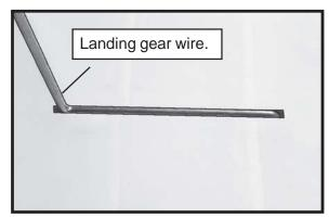
☐ 3) The landing gear wire is held in place using two nylon landing gear straps and four 3mm x 10mm wood screws.
