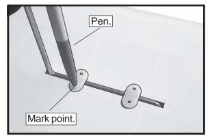
☐ 5) Remove the two straps and the gear wire. Drill four 1.5mm pilot holes into the wing for the wood screws.
