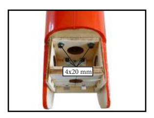
4) Attach the motor to the front of the electric motor box using four 4mm blind nut, four M3x15mm hex head bolts to secure the motor. Please see picture shown.
