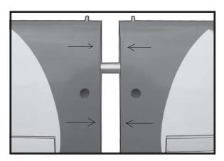
Apply masking tape at the wing join to hold the wing halves together securely.
