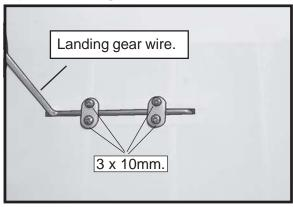
☐ 6) Reinstall the gear wire and install the straps using the four 3 x 10mm wood screws. Tighten the screws completely to secure the gear wire in place.
