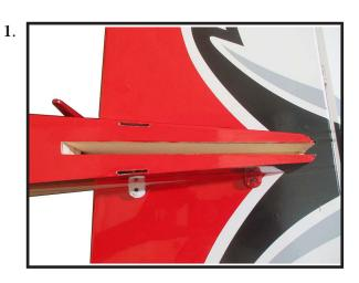
While holding the vertical stabilizer firmly in place, use a pen and draw a line on each side of the vertical stabilizer where it meets the top of the fuselage.
