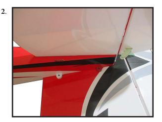
Thread the rudder cable through a brass swage tube, then the threaded co pler, and back through the brass swage tube on both sides. Pull light tension on the cable through the coupler on both sides as shown.
