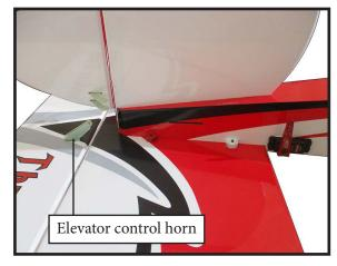
Thread one clevis and M3 lock nut on to each elevator control rod. Thread the horns on until they are flush with the ends of the control rods.
