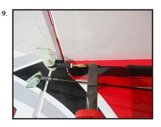
Cut off excess cable as shown.
