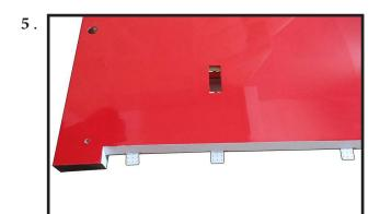
of the wing panels. Note the position of the hinges.
