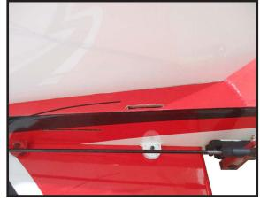
Thread cable through brass swage tube.
