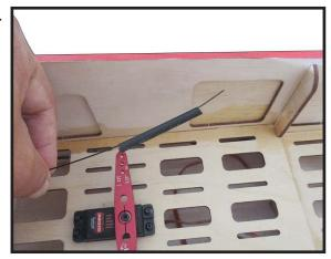
Thread cable through the threaded coupler hole, and back through the brass swage tube as shown.
