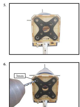
Then, use 3mm drill bit to enlarge the holes on the electric motor box.
