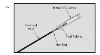
Use a felt tip pen to mark the wire where it crosses the hole. Use a pair of pliers to put a shrp 90-degree bend in the wire at the mark.
