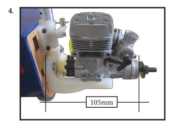
Use a pin drill and 3mm drill bit to drill a small indentation in the mount for the engine mounting screw.
