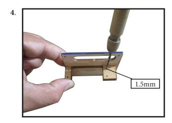
Apply 2-3 drops of thin C/A to each of the mounting holes. Allow the C/A to cure without using accelerator.
