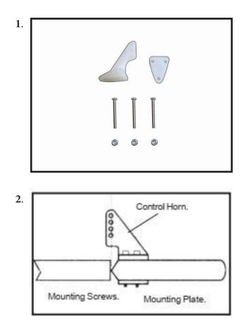
Using a 5/64" drill bit and the control horns as a guide, drill the mounting holes through the elevator halves.
