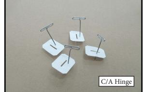
Remove each hinge from the wing panel and aileron and place a T-pin in the center of each hinge. Slide each hinge into the wing panel until the T-pin is snug against the wing panel. This will help ensure an equal amount of hinge is on either side of the hinge line when the aileron is mounted to the aileron.
