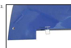
Slide the wing panel on the aileron until there is only a slight gap. The hinge is now centered on the wing panel and aileron. Remove the T-pins and snug the aileron against the wing panel. A gap of 1/64" or less should be maintained between the wing panel and aileron.
