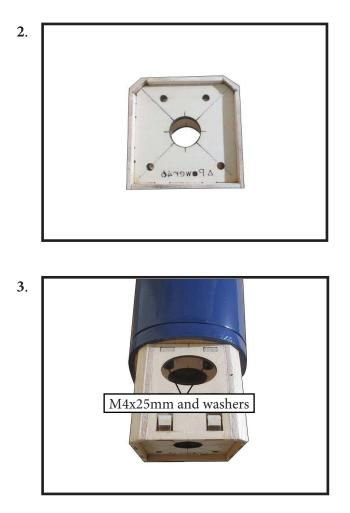
Attach the motor mount to the front of the electric motor box using four 4mm blind nut, four M4x25mm hex head bolts to secure the motor. Please see picture shown.
