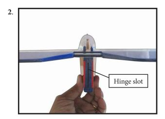
Slide the vertical stabilizer into the slot in the top of the fuselage. The rear edge of the stabilizer should be flush with the rear edge of the fuselage and the lower rudder hinge should engage the precut hinge slot in the lower fuselage. The bottom edge of the stabilizer should also be firmly pushed against the top of the horizontal stabilizer.
