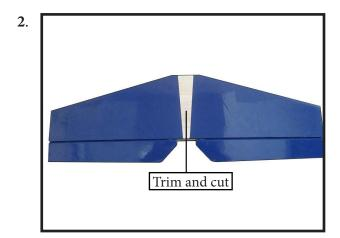
When cutting through the covering to remove it, cut with only enough pressure to only cut through the covering itself. Cutting into the balsa structure may weaken it. Using a modeling knife, carefully remove the covering that overlaps the stabilizer mounting platform sides in the fuselage. Remove the covering from both the top and the bottom of the platform sides.
