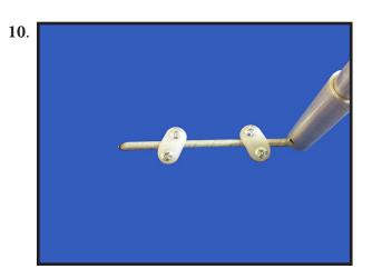
Reinstall the gear wire and install the straps using the four 3mm x 15mm wood screws. Tighten the screws completely to secure the gear wire in place.
