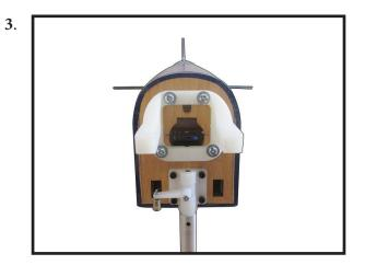
Position the engine with the drive washer (105mm) forward of the firewall as shown
