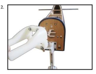
Use four 4x25mm head bolts and four 4mm washers to attach the engine mount rails to the firewall. Tighten the screws .Make sure to use threadlock on the screws to help prevent them from vibrating loose.
