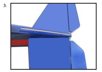
After the epoxy has fully cured, remove the masking tape or T-pins used to hold the stabilizer in place. Carefully inspect the glue joints. Use more epoxy to fill in any gaps that may exist that were not filled previously and clean up the excess using a paper towel and rubbing alcohol.
