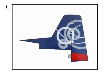
Using a modeling knife, remove the covering from over the precut hinge slocut into the lower rear portion of the fuselage. This slot accepts the lower rudder hinge.
