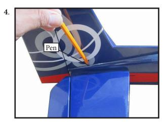
Remove the stabilizer. Using a modelling knife, remove the covering from below the lines you drew. Also remove the covering from the bottom edge of the stabilizer and the bottom and top edges of the filler block. Leave the covering in place on the sides of the filler block.
