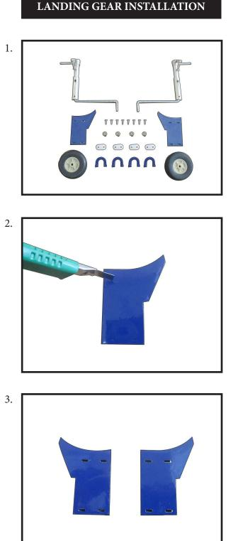
Using a modeling knife, remove the covering from over the two main gear mounting slots located in the bottom of the wing.
